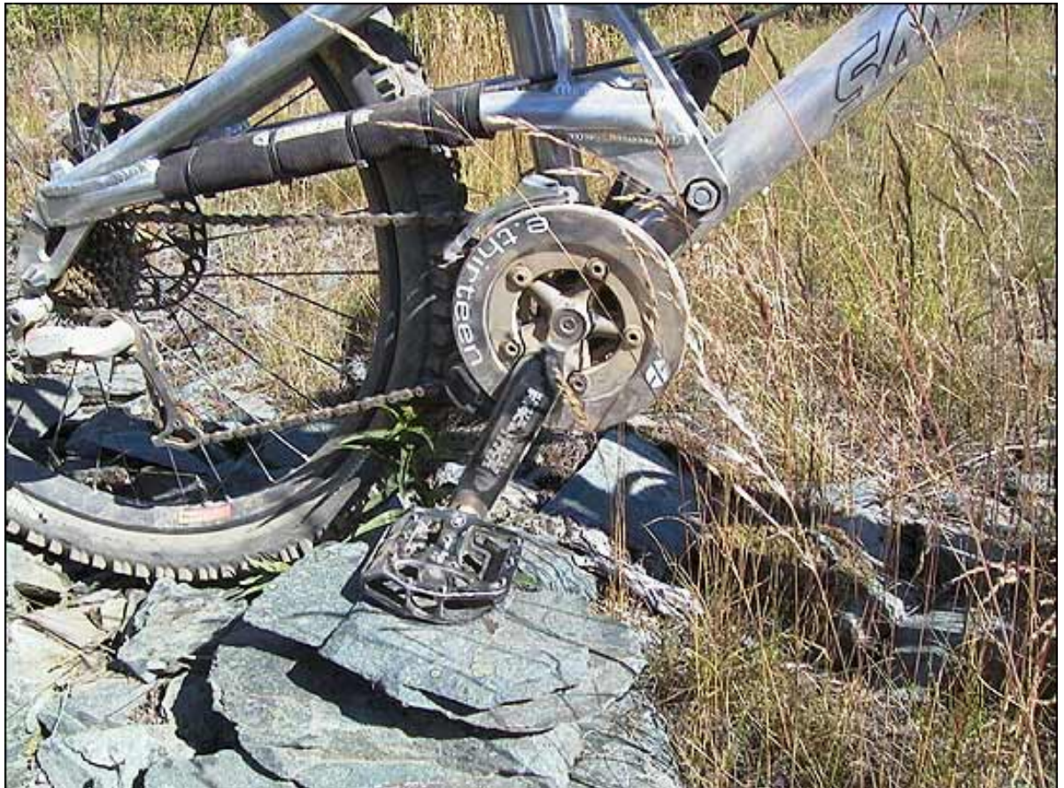
The DRS worked exceptionally well in dry and wet conditions - note the front derailleur
