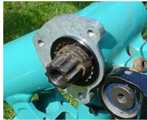
The plate mounts "flange side in" to the BB shell to give ISCG mounts.
