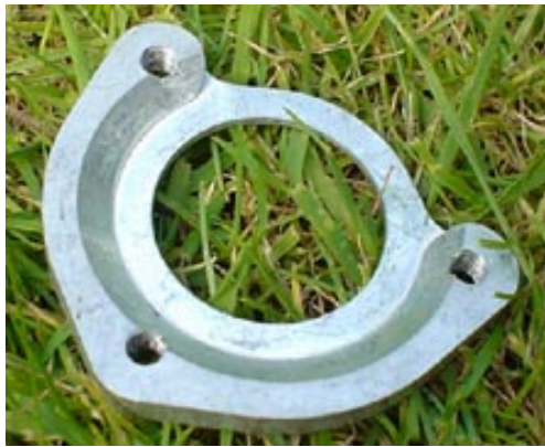
The plate mounts "flange side in" to the BB shell to give ISCG mounts.
